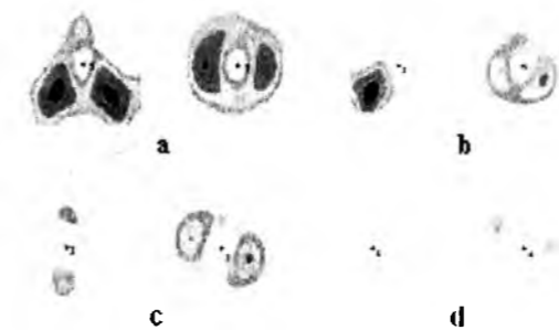
Fig.5. Sections in crossly perpendicular planes of the space valence electron density distribution for free-standing silicon wire in a neighbourhood of atoms of basis with numbers 1(a), 2(b), 3(c), 4(d)
